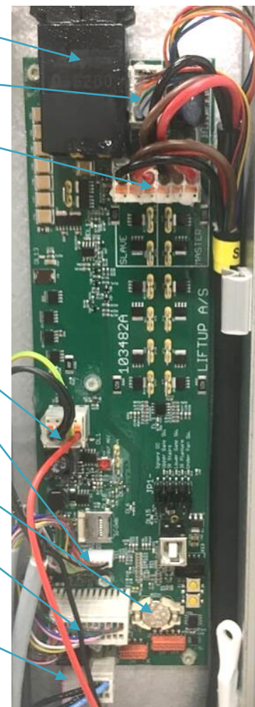
PRIMARY Control board (103482) RH side
