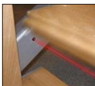
Infrared sensors prevent crushing between steps.
